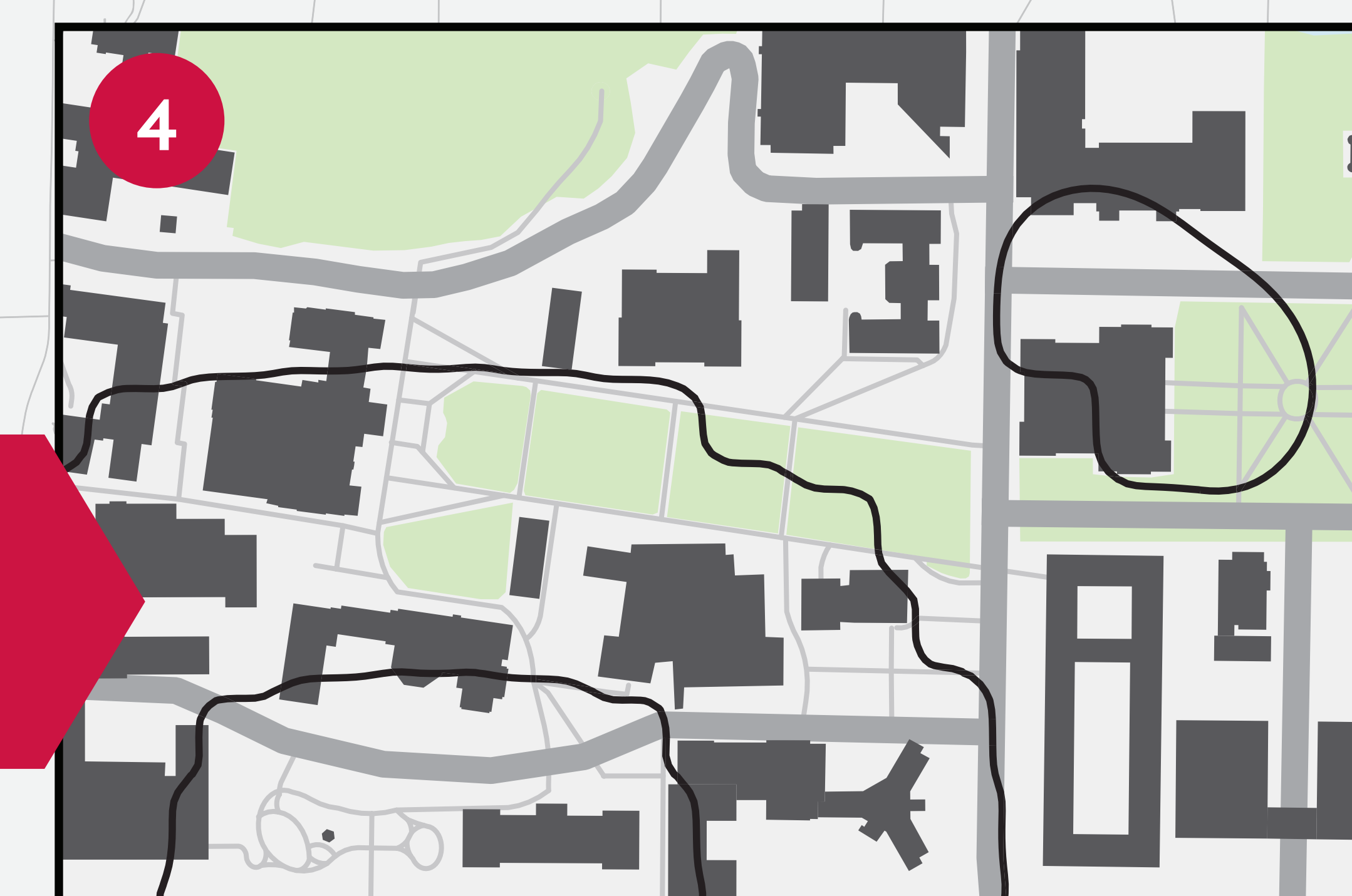
Finally, we use Inverse Distance Weighted interpolation (IDW) to generate contour lines at intervals useful for analysis. These can be saved as shapefiles for interactive visualization.
